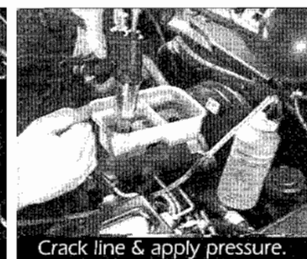
Crack line & apply pressure.
